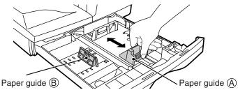
Fan the copy paper and insert it into the tray. Make sure the edges go under the corner hooks.
